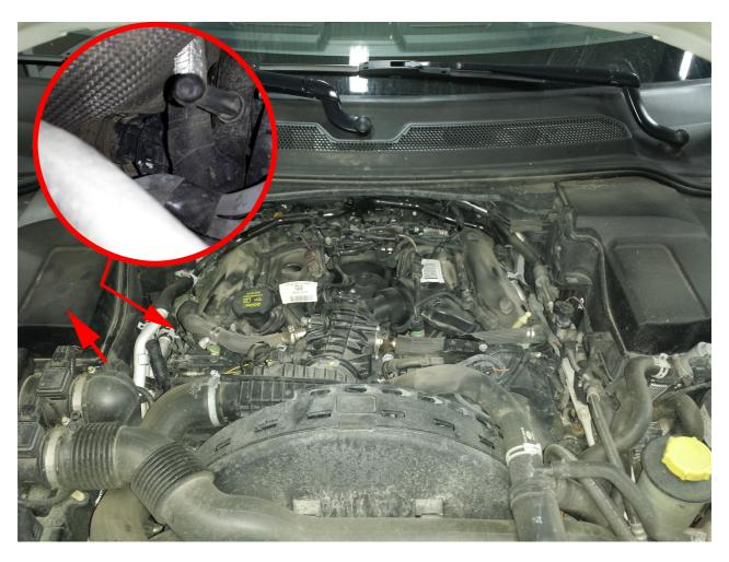
3. Connect yellow-red wire to positive terminal of a battery. It's easy to access after removing shield (arrow in the picture above).
