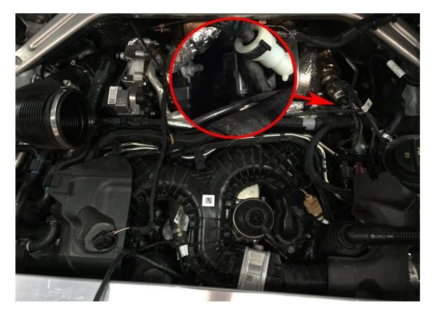
4. If box is equipped with yellow-red wire connect it to positive terminal in an engine compartment.
