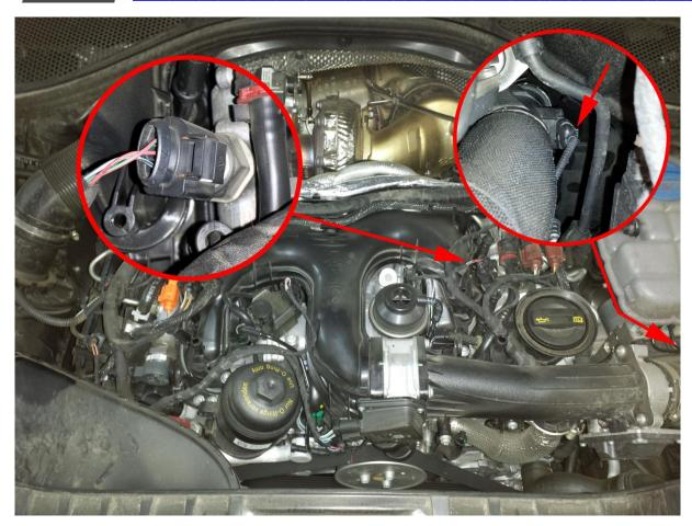
5. Connect yellow-red wire to positive terminal in an engine compartment.
