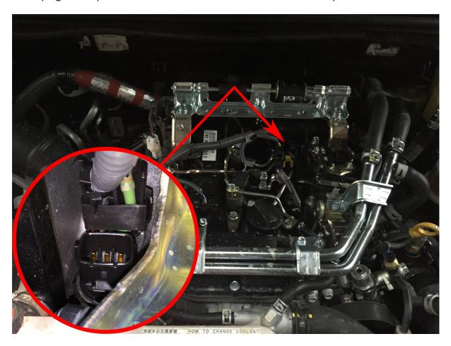
4. If box is equipped with yellow-red wire connect it to positive terminal in an engine compartment.
