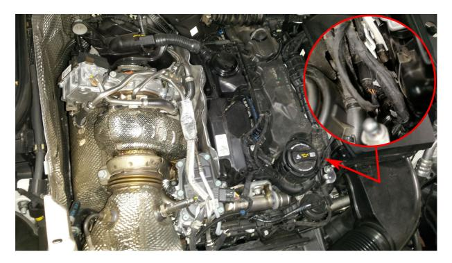
4. If box is equipped with yellow-red wire connect it to positive terminal in an engine compartment.
