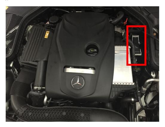
2. Switch ignition off, remove the key and wait about 5 minutes. Unplug ECU connectors and remove it from car.
