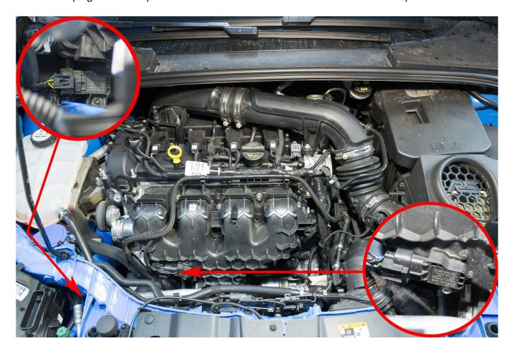
3. If box is equipped with yellow-red wire connect it to positive terminal in an engine compartment.
