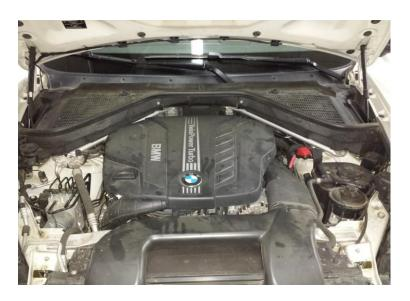
2. Remove the engine shield and air filter housing.
