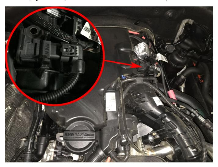
5. If box is equipped with yellow-red wire connect it to positive terminal in an engine compartment.
